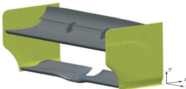
Figure 29. Wings of a race car [29].
