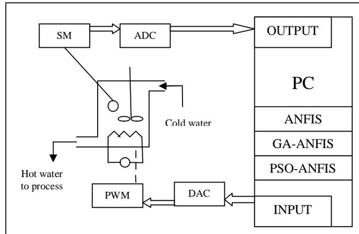
Figure 6: Schematic diagram of Water bath temperature control system
