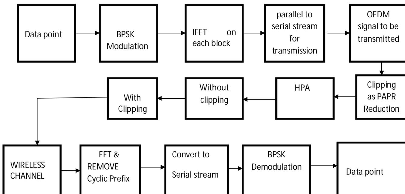
Figure.3 OFDM Transmitter & Receiver
