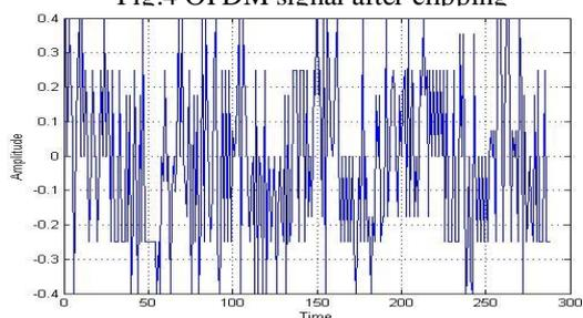
Fig.7 With Clipped OFDM signal after HPA
