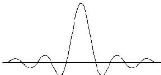
Fig.1 Spectrum of an OFDM Sub-channel
