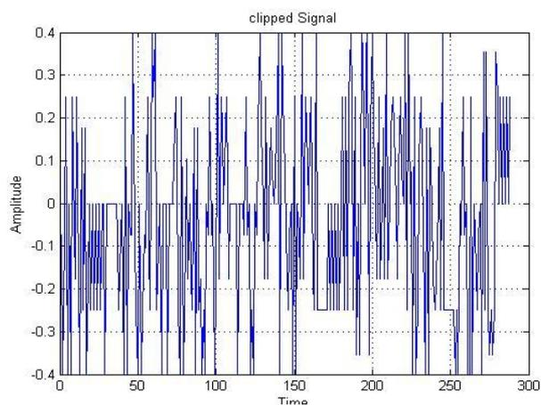
Fig.4 OFDM signal after clipping
