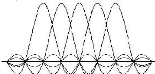
Fig.2 OFDM Spectrum (During a signal bit)
