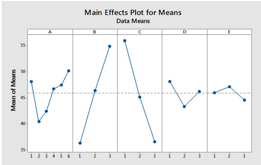
Figure1. Main Effect Plot for S/N ratio and MEAN for material removal rate
