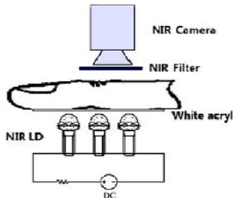
Finger vein reader consists of IR LED, Webcam and adapter. Adapter provides power supply to the IR LED. IR LED is placed below the finger and Webcam is placed above it. IR LED provides light source to the finger which reflects the inner part of finger which is enough to capture vein image with high resolution. Webcam captures the finger image and gives this image to laptop as input. Then further process of like preprocessing and segmenting are done using software such as MATLAB.
