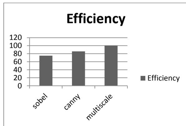
Figure 9: Comparison of Efficiency of Canny and Sobel with wavelet edge detection techniques
