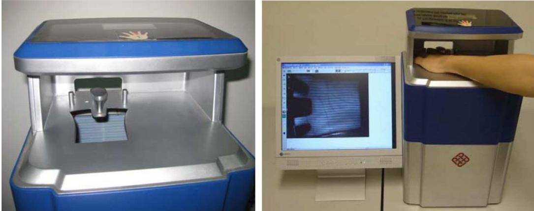
Fig. 1. Developed palm print authentication system with structured light imaging and an example of the use of the system.
