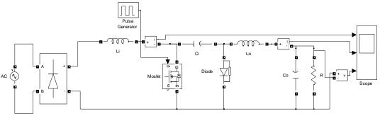
Fig. 4 Simulink model of open loop non- isolated Cuk converter
