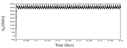
Fig.5 Open loop response of non-isolated Cuk converter
