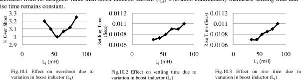
Fig.10 Effect on inductor current (IL<sub>0</sub>) due to variation in boost inductor (L<sub>i</sub>)
