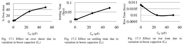
Fig.17 Effect on output voltage  $(V_0)$  due to variation in filter capacitor  $(C_0)$
