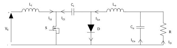
Fig. 1 Schematic diagram of non-isolated Cuk converter
