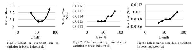
Fig.8 Effect on output voltage (V<sub>0</sub>) due to variation in boost inductor (L<sub>i</sub>)
