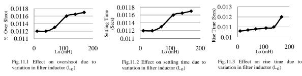
Fig.11 Effect on output voltage (V<sub>0</sub>) due to variation in filter inductor (L<sub>0</sub>)
