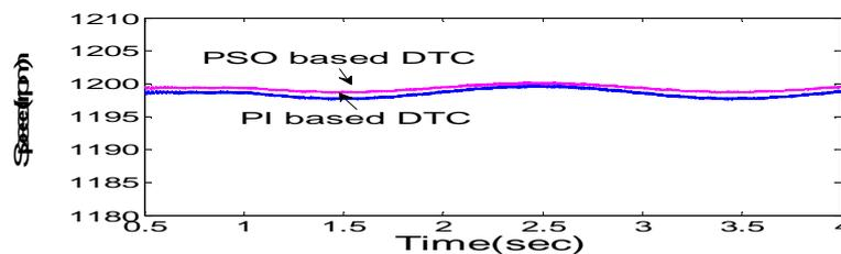
Fig.7 (b) Speed comparison with conventional and PSO based DTC
