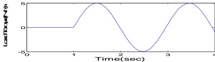
Fig.7 (a) External load torque disturbance
