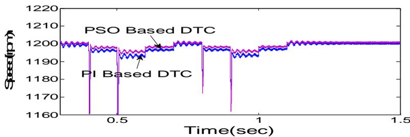
Fig.5 (b) Speed comparison with conventional and
