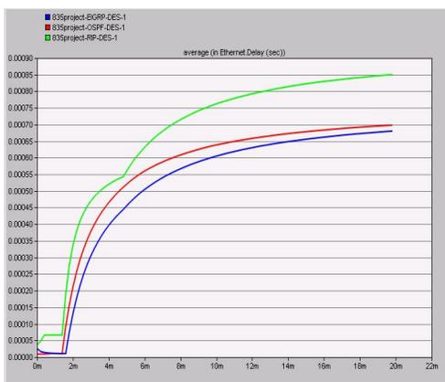
Fig. 4 Performance based on Ethernet delay
