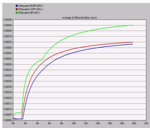
Fig. 4 Performance based on Ethernet delay
