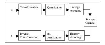
Figure 2. Block diagram of DWT based Compression Scheme
