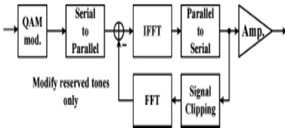
Fig. 1. Iterative FFT/IFFT processing for tone reservation
