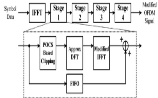
Fig 2. Proposed structure for the tone reservation method
