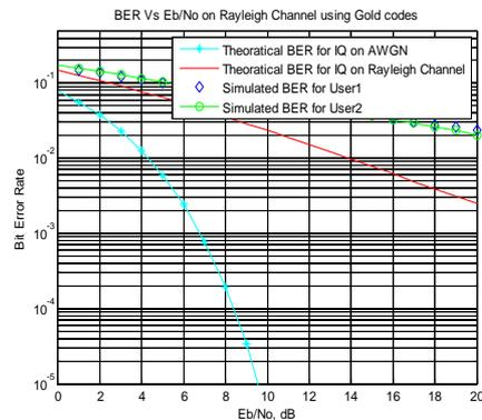
Fig 3.6 Graphs obtained after performance of system using GOLD code
