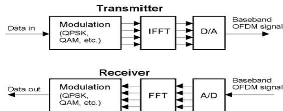
Fig 2.1 Block diagram of OFDMA Transmitter and Receiver
