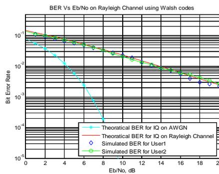
Fig 3.4 Graphs obtained after performance of system using WALSH code
