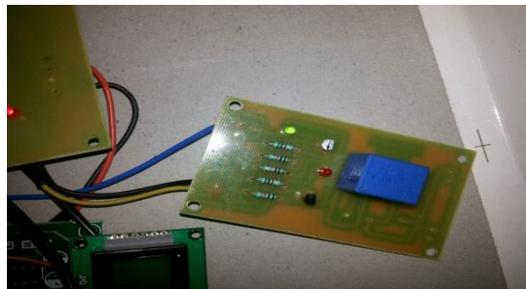
Figure 9: Power Supply board
