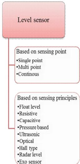
Figure 5: Level sensor types
