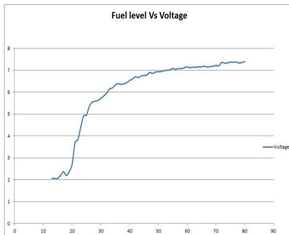
Figure 8: Fuel level sensor output
