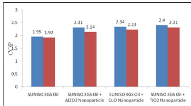
**FIG.4. COMPARISON OF COP FOR THE FOUR CASES**
