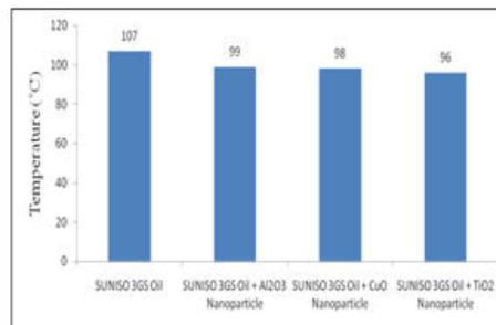
**FIG.6. TEMPERATURE OF THE COMPRESSOR DOME**
