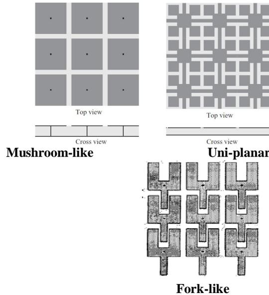
Fig 1. Various types of EBG structure
