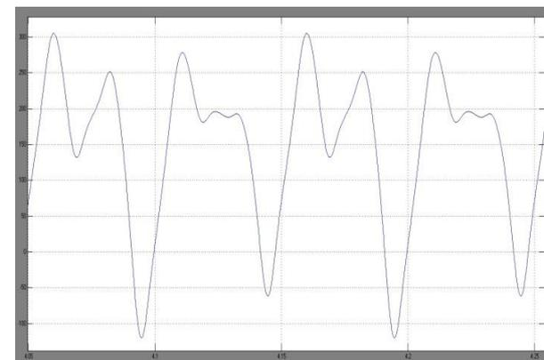
Figure 13: Speed waveform (Period Five) for 140 Volt (R.M.S)
