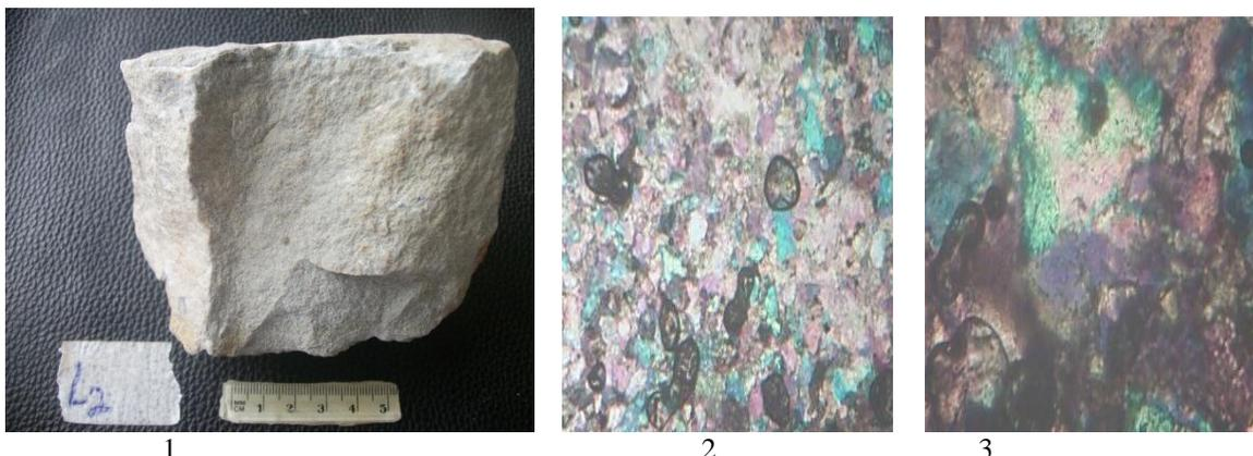
**1.** Hand specimen of sandstone. **2** Photomicrographs of 1 showing Quartzo-feldspathic hornfels,. Note alignment and elongation of minerals top to bottom, vertically. The irregular dark grains are hornblende. There are also biotite and iron ore.
