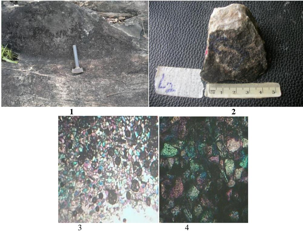
**1.** Calcareous Sandstone, quarry site at location .2 along Amasiri-Ozara Ukwu Road: Calcareous Sandstone, quarry site at location 2 along Amasiri-Ozara Ukwu Road. **3 & 4** Photomicrographs of Buchite hornfels,. Note speckles of magnetite minerals and a granoblastic mosaic of quartz and feldspars, with web texture.
