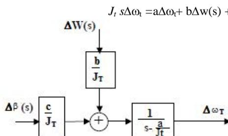
The linear turbine model is as shown in figure (2) where
