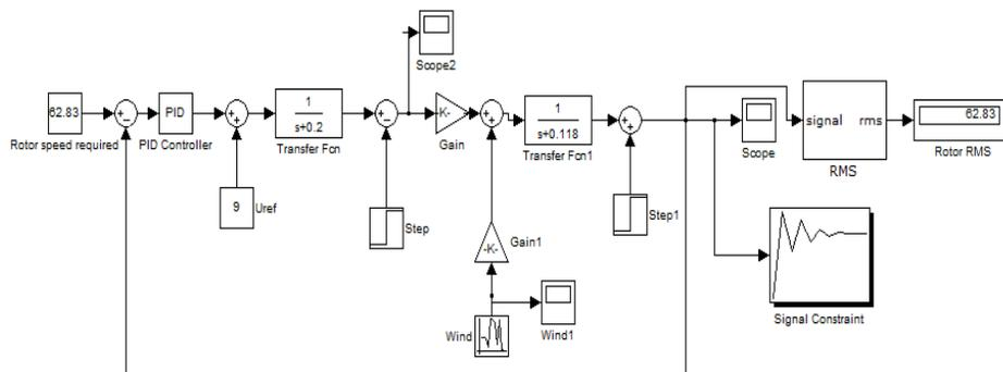
Figure 6. Simulink Block Diagram
