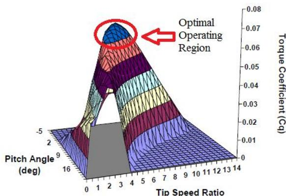
Fig 1. Power coefficient surface as a function of tip-speed ratio and blade-pitch angle.
