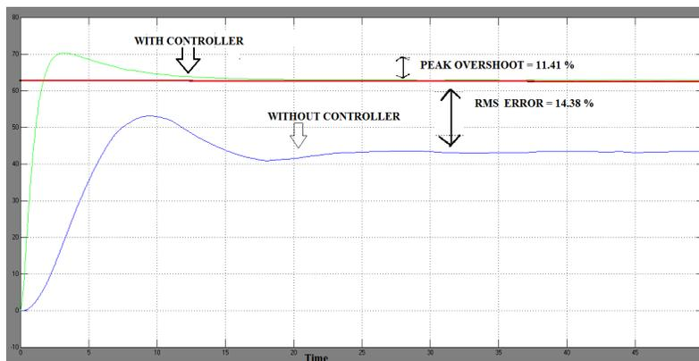
Figure 9. Rotor Speed output using manual tuning of the PID controller
