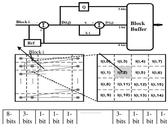
**Fig2.** Architecture of the block buffer
