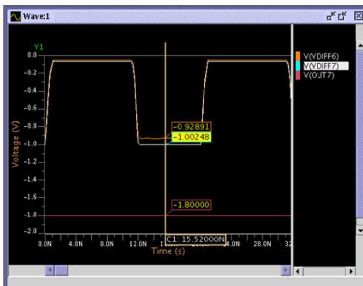
**Fig4.** Pixel 7 outputs, where  $V_{diff6}$  and  $V_{diff7}$  are inputs to comparator of pixel 7 and  $V_{out7}$  is output of pixel 7.
