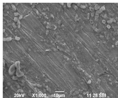
Figure 6: SEM image of EBAP MMT
