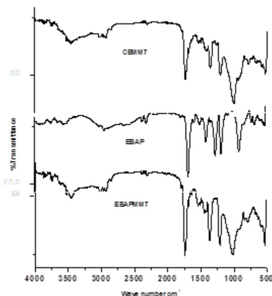
Figure 1: IR spectra of cationic exchange MMT (CEMMT), EBAP and the composite EBAPMMT
