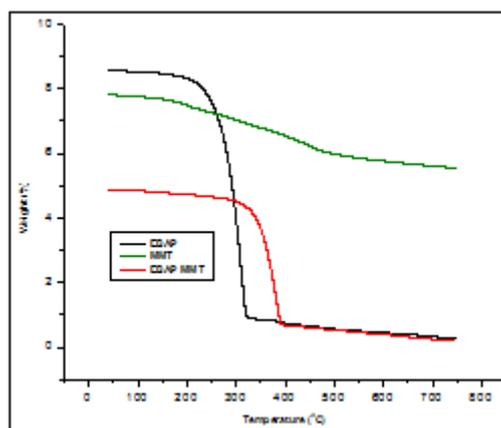
Figure 4: TGA curves of polymer, MMT and Composite
