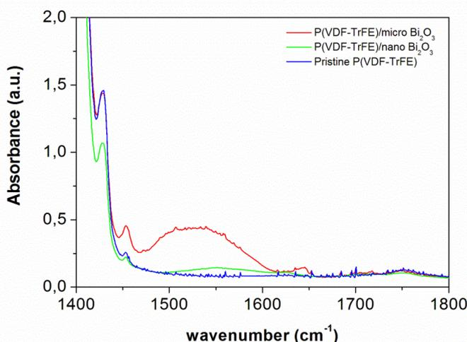
**Figure 6:** FTIR spectra of P(VDF-TrFE) copolymer and P(VDF-TrFE)/Bi<sub>2</sub>O<sub>3</sub> nano and microcomposites for wavenumbers ranging from 1400 cm<sup>-1</sup> to 1800 cm<sup>-1</sup>.
