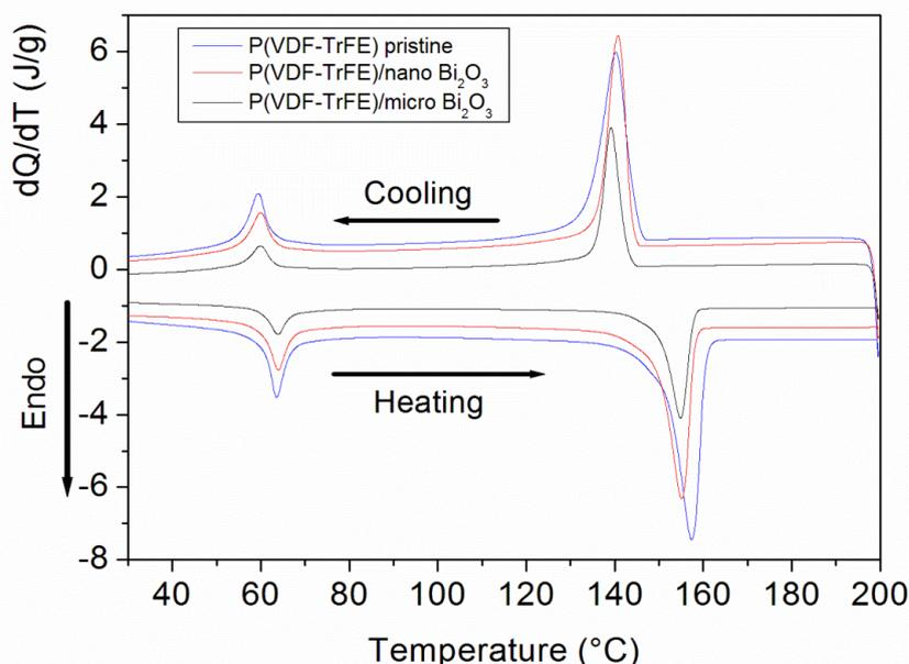
**Figure 5:** DSC thermograms of P(VDF-TrFE) copolymer and of P(VDF-TrFE)/Bi<sub>2</sub>O<sub>3</sub> nano and microcomposites, collected at the 2<sup>nd</sup> heating/cooling run.
