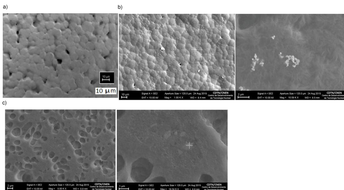
**Figure 3:** (a) SEM images taken on the surface of P(VDF-TrFE) pristine sample magnified 1310x (b) P(VDF-TrFE)/ $\text{Bi}_2\text{O}_3$  nanocomposite magnified 1000x (left side) and 1050x (right side) and (c) P(VDF-TrFE)/ $\text{Bi}_2\text{O}_3$  microcomposite magnified 5000x (left side) and 1834x (right side). The white cross mark on images [(b) and (c) left] correspond to the points where the EDS probe was pointed in order to measure the presence of  $\text{Bi}_2\text{O}_3$  material.
