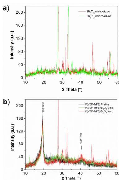
**Figure 4:** a) Diffractograms of nano and micro crystalline Bismuth Oxide and b) diffractograms of pristine P(VDF-TrFE) copolymer and its composites with nano and microsized Bi<sub>2</sub>O<sub>3</sub>.
