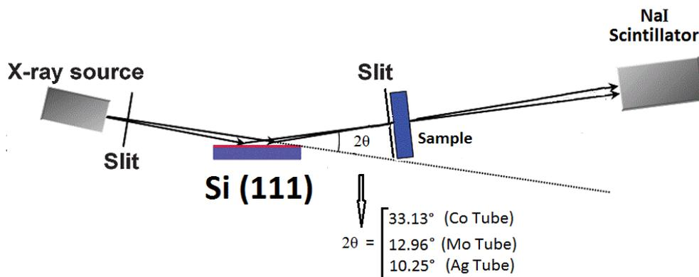
**Figure 1:** Schematic diagram of the setup used to irradiate P(VDF-TrFE)/ $Bi_2O_3$  samples with monoenergetic X-rays using Co, Mo and Ag tubes with photons of 6.5 keV, 17,5 keV and 22,1 keV, respectively.
