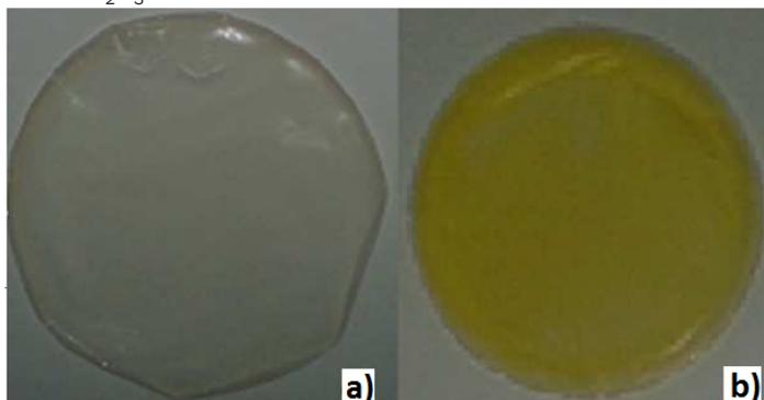
**Figure 2:** Photographs taken just after the complete evaporation of a typical P(VDF-TrFE)/ $\text{Bi}_2\text{O}_3$  film sample prepared with a) 8 wt% of  $\text{Bi}_2\text{O}_3$  microparticles and b) 8 wt% of  $\text{Bi}_2\text{O}_3$  nanoparticles.
