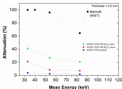
**Figure 8:** X-ray beam attenuation of P(VDF-TrFE) copolymer and P(VDF-TrFE)/ $\text{Bi}_2\text{O}_3$  nano and microcomposites as a function for 33 keV, 54 keV and 83.5 keV mean energies of the X-ray beam qualities RQR2 (40 kV), RQR5 (70 kV) and RQR 8 (100 kV). The thickness sample was normalized to 0.5 mm
