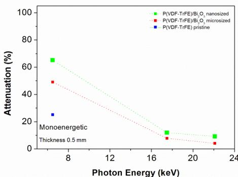
**Figure 7:** X-ray beam attenuation of P(VDF-TrFE) copolymer and P(VDF-TrFE)/ $\text{Bi}_2\text{O}_3$  nano and microcomposites as a function for 6.6 keV, 17.5 keV and 22.1 keV monoenergetic photons. The thickness sample was normalized to 0.5 mm.
