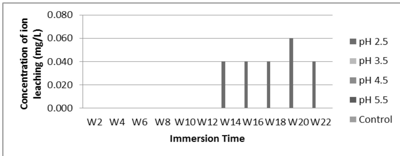
**Figure 1.** Silver ion leaching from transpalatal arch (TPA) immersed in hydrochloric acid of different pH and control as expressed in mg/L. ('Control' used in this study was deionised distilled water).
