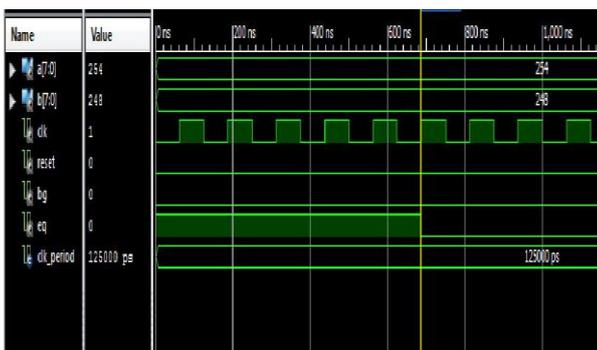
**Figure 5:** Output of comparator using Binary Tree Architecture.
