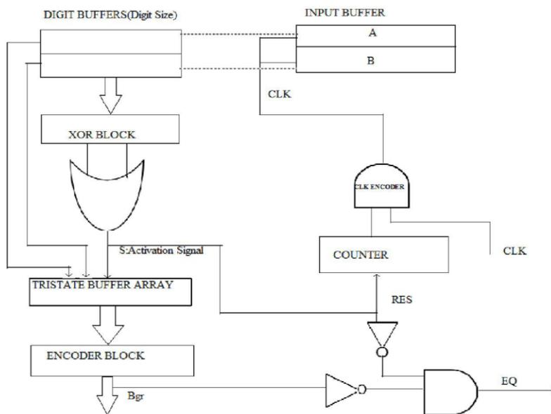
Figure 2: Block diagram of comparator.
