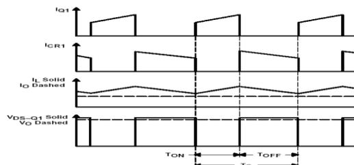
Fig.3. Continuous mode Boost power stage waveforms
