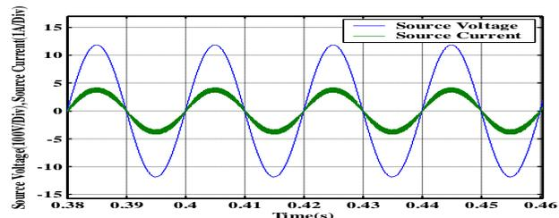
Fig. 4.5 Source current and voltage waveforms of the Boost Rectifier switched by the PSM at R=350Ω
