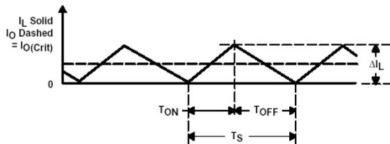
Fig. 4(a)Boost Converter at the boundary of Continuous-Discontinuous Conduction
