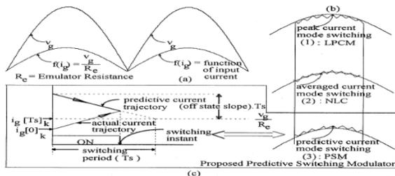
Fig. 16 Generalized control objective of the carrier-based current mode controllers
