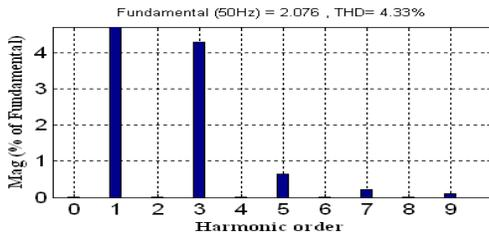
Fig. 4.4 Harmonic spectrum of the source current at R=650Ω
