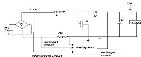
Fig. 10 Block diagram of PFC circuits at CCM operation with the Multiplier approach
