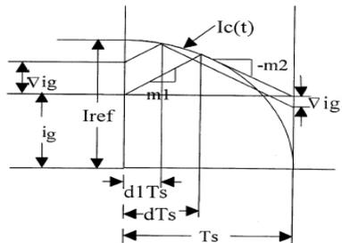
Fig.18 (a) Carrier Waveform of the PSM,
