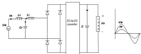
Fig. 9 The active power factor correction Technique the Multiplier approach
