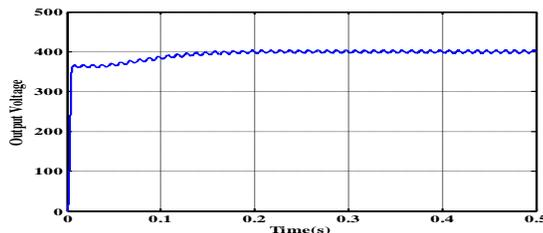
Fig. 4.6 Output voltage waveforms of the boost rectifier switched by the PSM at R=350Ω
