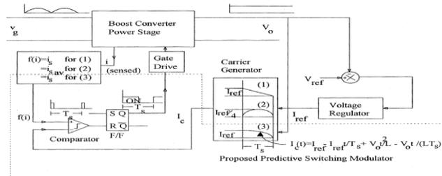
Fig. 17 Block Diagram of the carrier based input-current-shaping controllers: (the LPCM; 2) the NLC 3) the PSM
