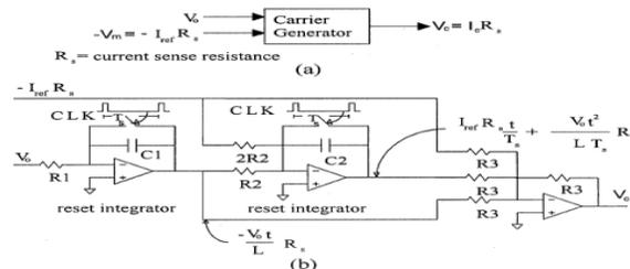
Fig. 23.(a) Carrier generator block of the PSM., (b) Circuit realization
