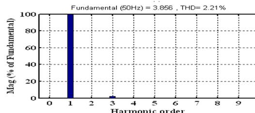
Fig. 4.7 Harmonic spectrum of the source current at R=350Ω
