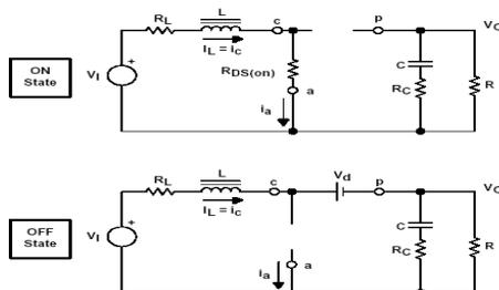
Fig.2.Boost power stage stages
