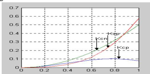
Fig. 20. Comparison of different critical k parameters: 1)  $K_{sp}$  steady state stability condition with the PSM; 2)  $K_{cp}$ : CCM operation with the PSM; and 3)  $K_{cn}$  CCM operation with the NLC.
