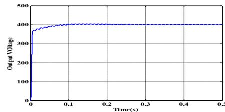
Fig. 4.3 Output voltage waveforms of the boost rectifier switched by the PSM at R=650Ω. For 650 ohms of resistance, source voltage and source currents are as shown in fig. 4.2 above
