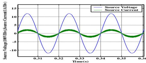
Fig. 4.2 Source current and voltage waveforms of the Boost Rectifier switched by the PSM at R=650Ω. For 650 ohms of resistance, output voltage waveforms are as shown in fig 4.3 above
