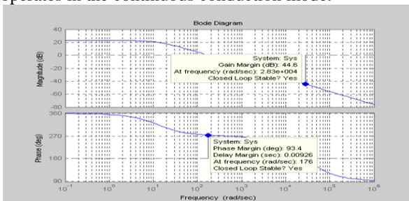
Fig. 22. Bode plot of the control gain transfer function  $G_v(s)$  of the PSM switched boost rectifier
