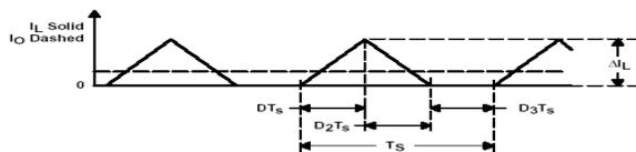
Fig. 5.Boost Converter Waveform at Discontinuous Conduction
