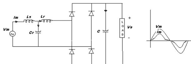
Fig. 8. The Passive Power factor correction technique
