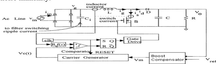
Fig. 15. Power circuit of the single phase PFC rectifier with the generalized control structure of the NLC, the LPCM, and the PSM.
