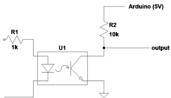
Figure 6: Optocoupler circuit.
