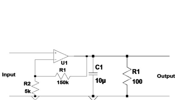
Figure 5: Receiver Amplifier and Envelop Detector.
