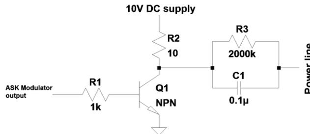
Figure 1: Power Amplifier and Coupling Circuit.
