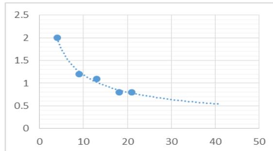
Figure 7: Variation of signal level (V) with distance (m).
