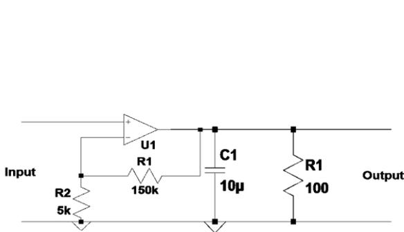
Figure 5: Receiver Amplifier and Envelop Detector.
