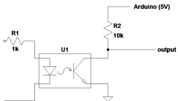
Figure 6: Optocoupler circuit.
