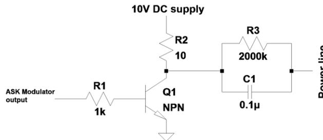
Figure 1: Power Amplifier and Coupling Circuit.
