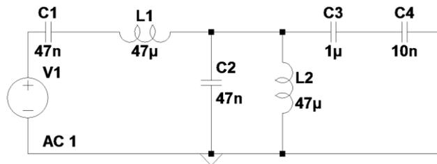
Figure 2: Receiver Coupling Circuit.
