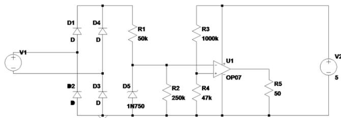
Figure 2: Zero Crossing detector.
