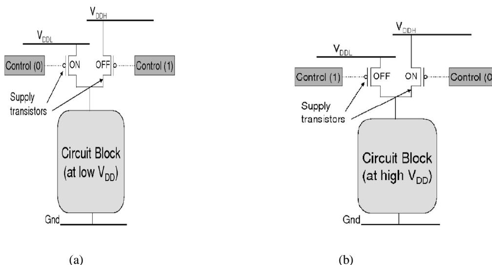
Figure 3.1 Supply Transistors used for programmable  $V_{DD}$
