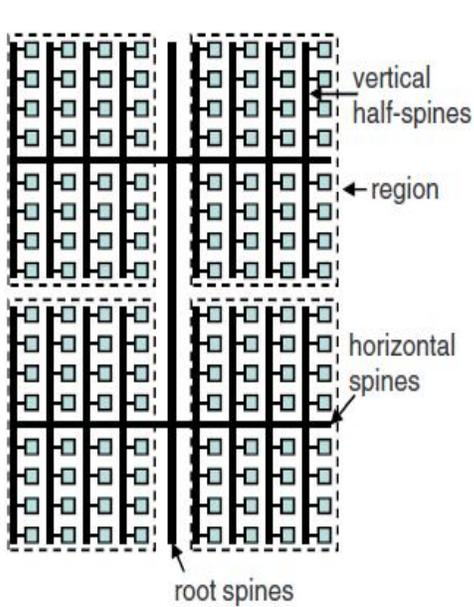
Figure 2.1 Coarse grained Architecture
