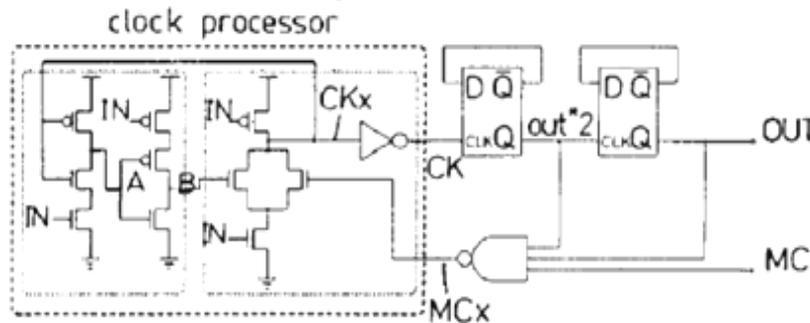
Fig.2. Schematic diagram of circuit of divide-by-4/5
