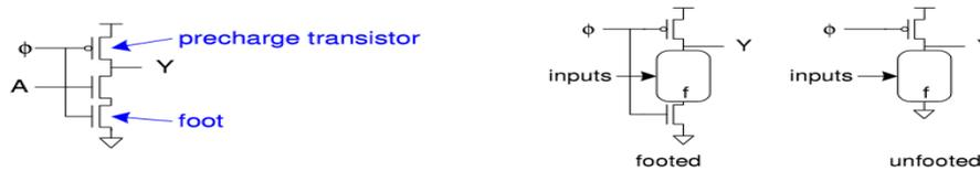
Fig.1. Logic diagram of Footed Technique
