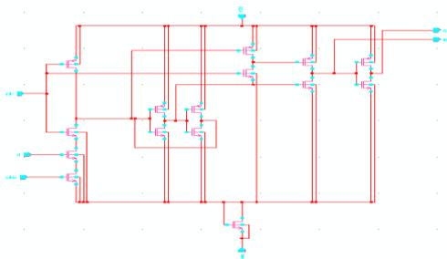
Fig.7.Schematic Diagram of Proposed DDFD with footed logic
