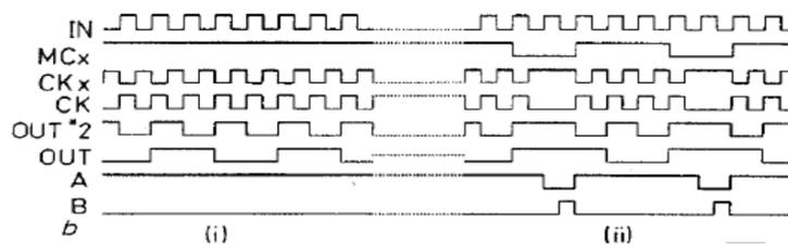
Fig.3. Timing diagram divide-by-4/5
