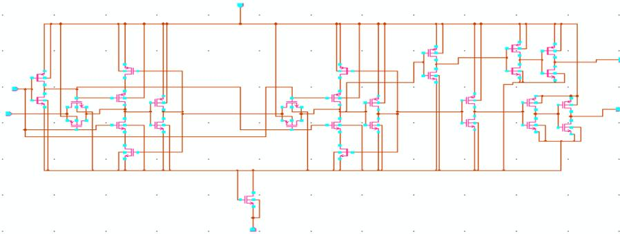
Fig.4.Schematic Diagram of Power PC 603 Flip Flop with Footed Logic
