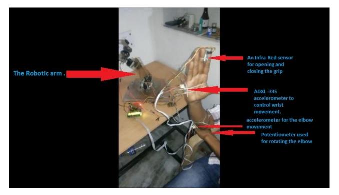
Figure 1. The complete setup including the robotic arm and the sensor setup that is worn around the human hand.
