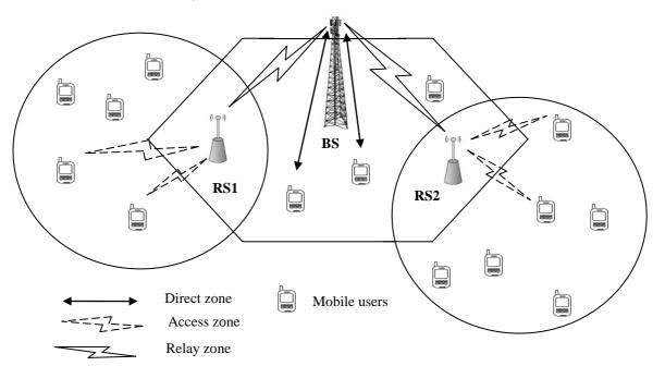
Fig. 1. Structure of WiMAX relay network
