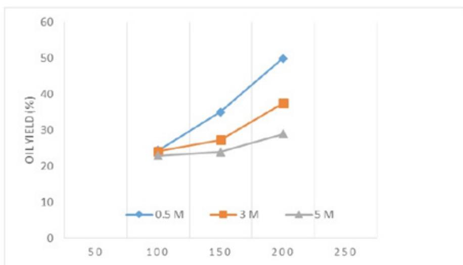
**Figure 4.** Yield algae oil extraction process (osmotic) using solvents HCl obtained at various volume HCl with stirring time of 3 hours.
