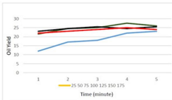
**Figure 3.** Algal oil yield (%- weight) of the extracted (osmotic) using a variety of solvents HCl molarity and stirring time is different.
