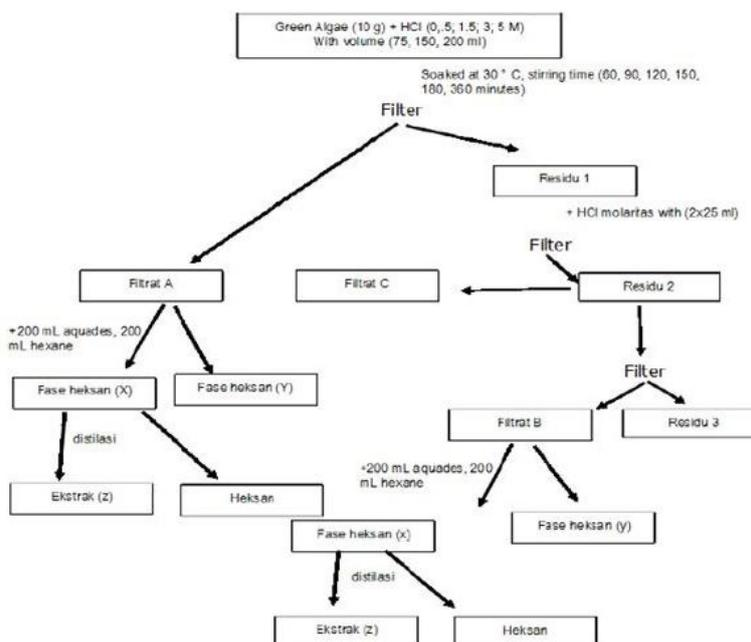
Figure 1. Flow diagram osmotic methods with solvents HCl.
