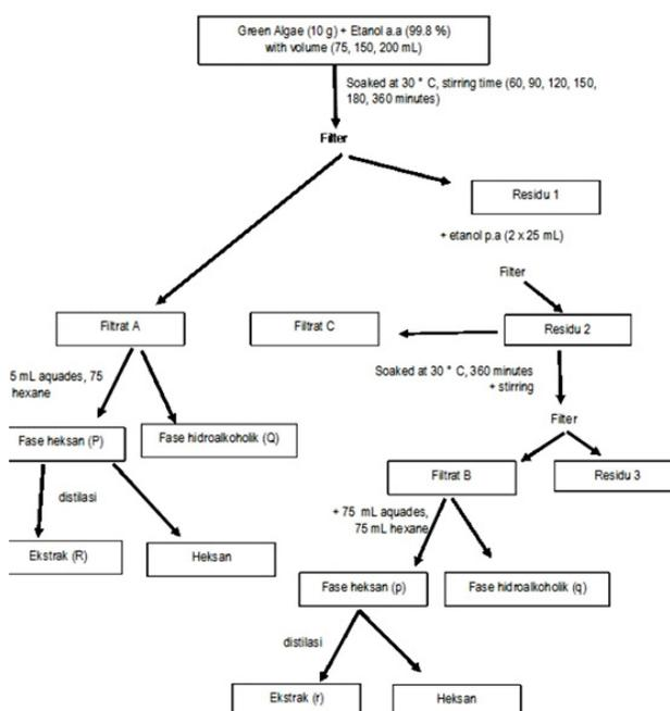
Figure 2. Flow diagram osmotic methods with solvents ethanol (99.8%).
