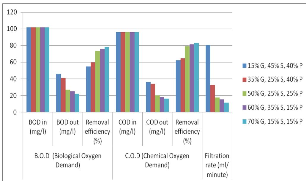
Figure 4: Biological oxygen demand (BOD) and Chemical Oxygen demand (COD) before and after filtration of the effluent. (G= Garden Soil S= Sand P =Pebbles)
