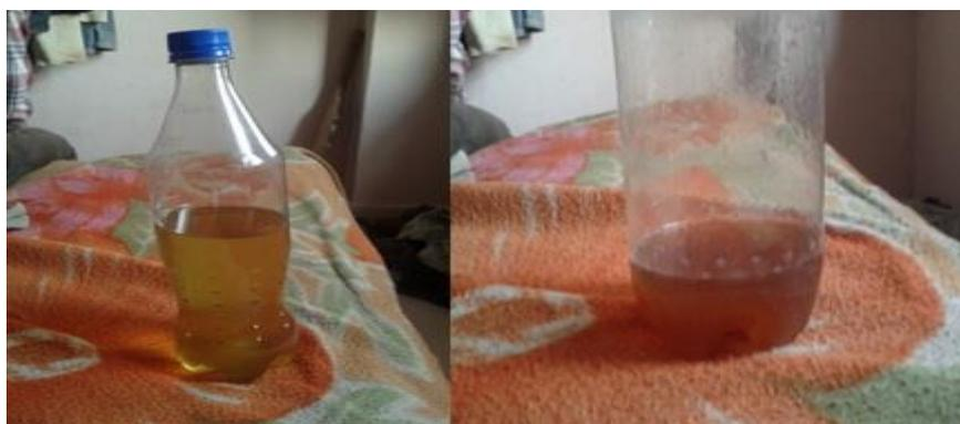
**Figure 6.** Separated biodiesel and glycerol from mixture.
