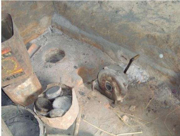
Fig 2 : Melting Pit Furnace ("Bhatta")
