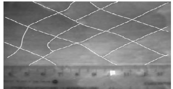
Fig .4 Soot foil imprint of detonation wave
