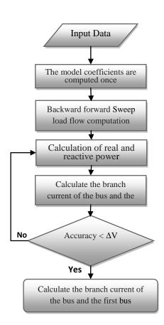
Figure 2: Flowchart of the proposed power flow
