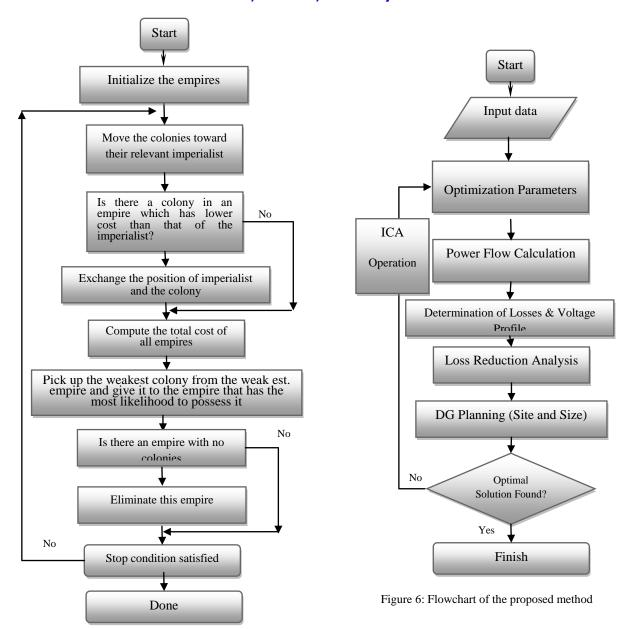
Figure 5: Flowchart of the proposed ICA algorithm
