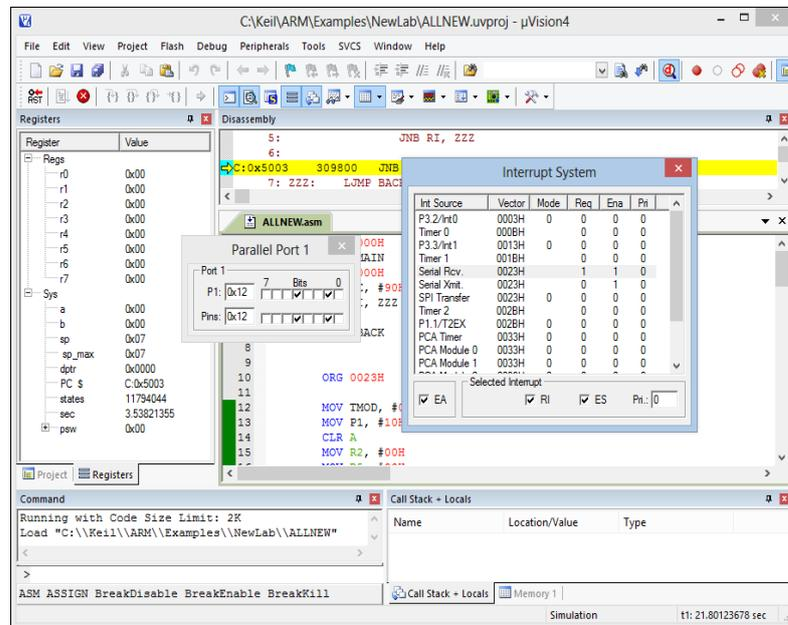
Fig. 8: Output of Keil simulator shown above indicates that now viewer is much closer to the television and so a warning alarm is switched on after approximately 30 seconds (Pin 4=TV, Pin 1=Alarm).
