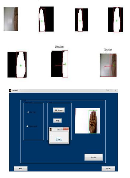
Fig .7 .The Gesture Recognition Hand Tracking System.(a) hand tracking system,(b) gesture recognition.
