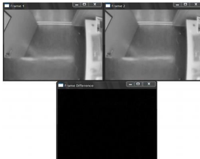
Fig. 2 Frame Differencing Algorithm Having No Motion
