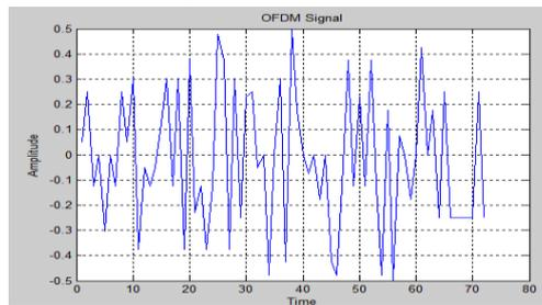
Figure 8: OFDM signal with QPSK
