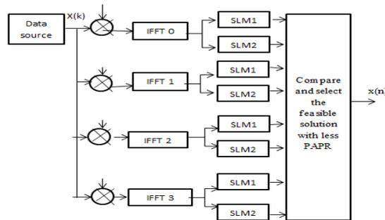
Figure3: OFDM System for IFFT calculation
