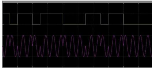
Figure 7: BPSK modulation
