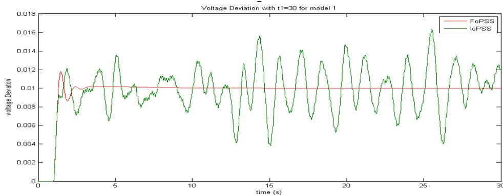
Fig 4 Voltage deviation without an AVR when  $D = 2, \tau_1 = 30, \tau_2 = 1$
