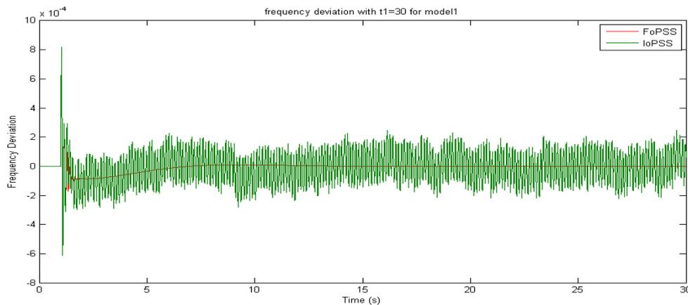
Fig 2 Frequency deviation due to 0.05 p.u. step change in both  $V_{ref}$  and  $T_m$  when  $D = 2$ ,  $\tau_1 = 30$ ,  $\tau_2 = 1$
