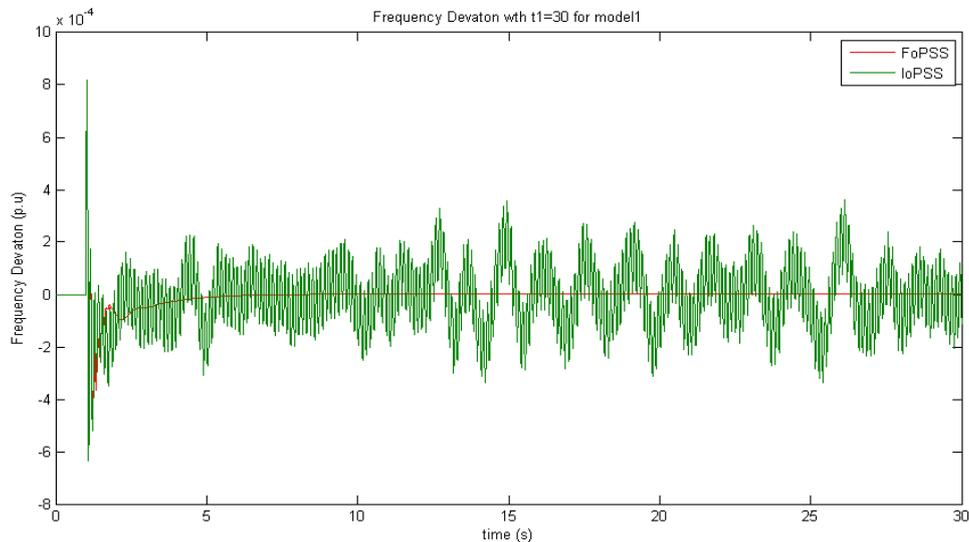
Fig 3 Frequency deviation without an AVR when  $D = 2, \tau_1 = 30, \tau_2 = 1$
