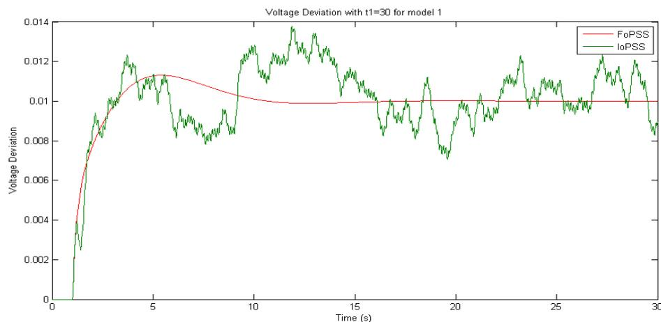
Fig 3 Voltage deviation due to 0.05 p.u. step change in both  $V_{ref}$  and  $T_m$  when  $D = 2$ ,  $\tau_1 = 30$ ,  $\tau_2 = 1$
