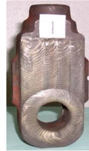
Figure 2 Typical Hardfaced Gate Valve having Linear and Circular Overlay Beads
