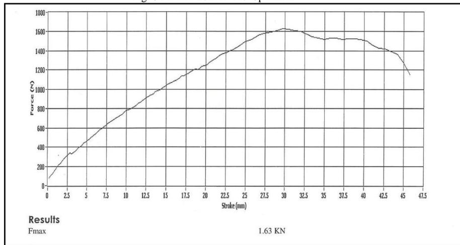
Fig. 9 Force versus displacement diagram to find out flexure strength
