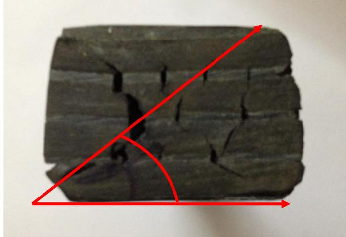
Fig. 6 Failed Edges of the Specimen.
