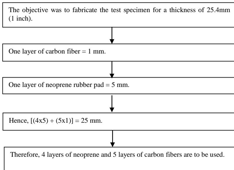
Fig. 1 Flowchart for the calculation of the number of layers to be used.
