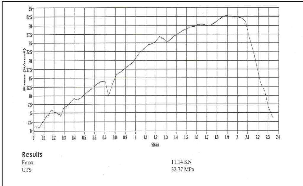
Fig. 4 Stress-Strain plot of the composite material under tension test.
