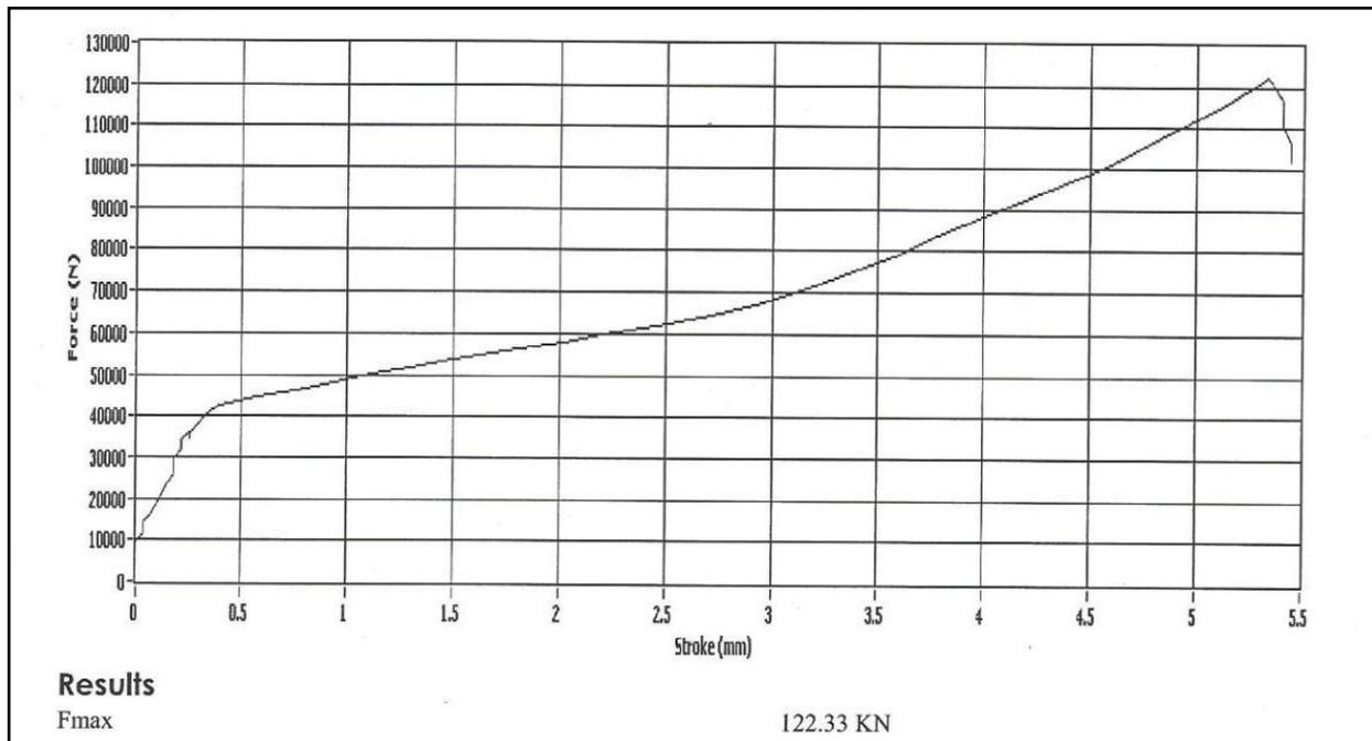
Fig. 7 Force versus displacement diagram to find compression strength
