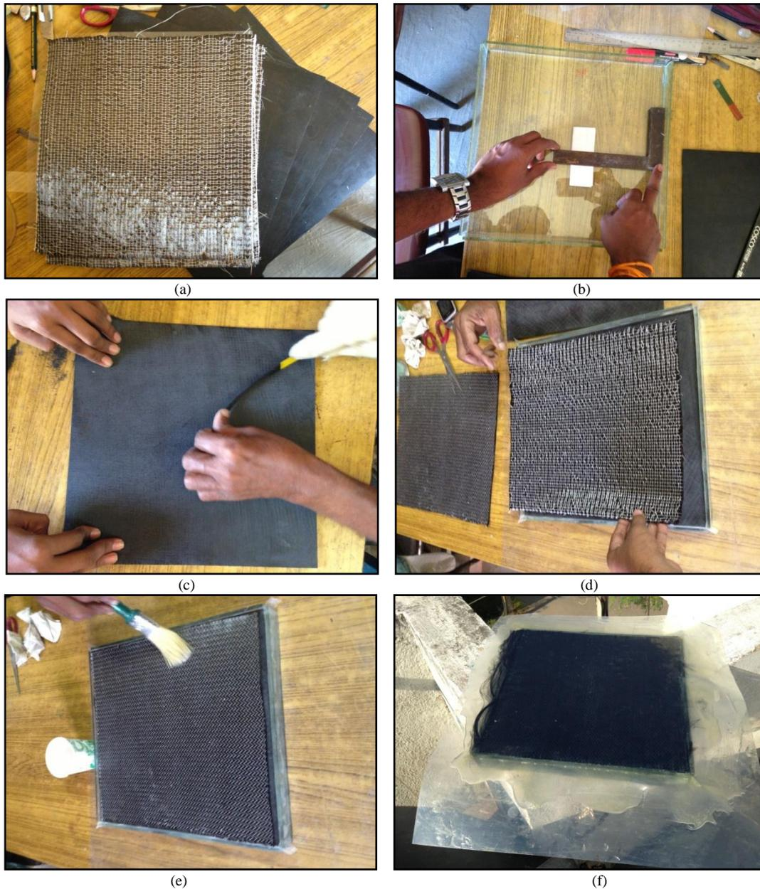
Fig. 3 Steps followed in fabrication of the material for test specimen (a) Cut Specimen (b) Perpendicularity Check (c) Scratch of the Specimen (d) Orientation of Fibers (e) Epoxy Resin Coating (f) Sun Dried Specimen.
