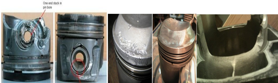
defect types (damages at Circlip groove, damage at crown head, damages at fixture seat)
