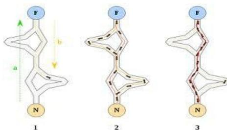
Fig. 1: All ants take the shortest path after an initial searching time.
