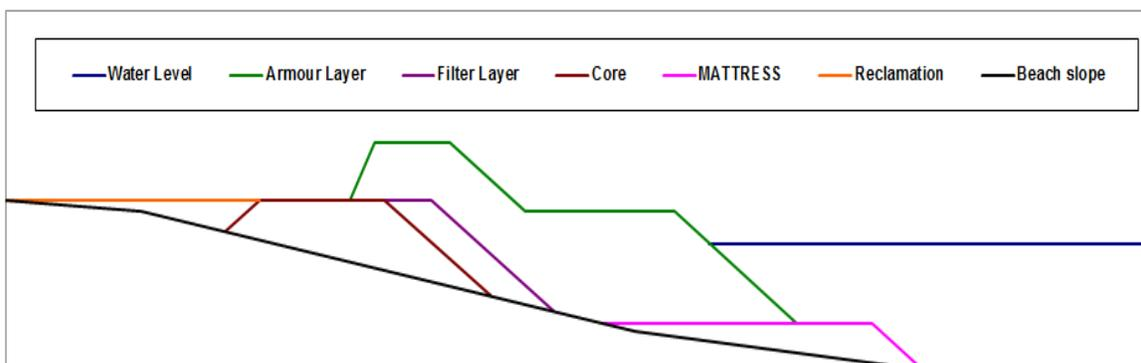
Figure 1: Design of the berm reshaped seawall
