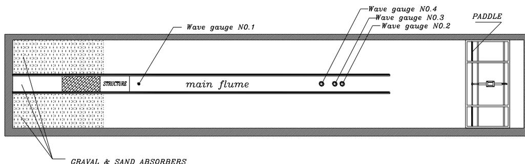
Figure 2: Plan view of the wave flume and setup of wave height meters
