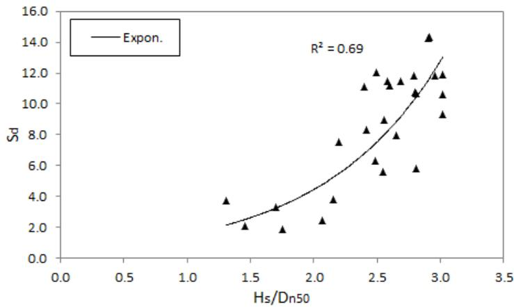
Figure 5: Damage parameter diagram against significant wave height
