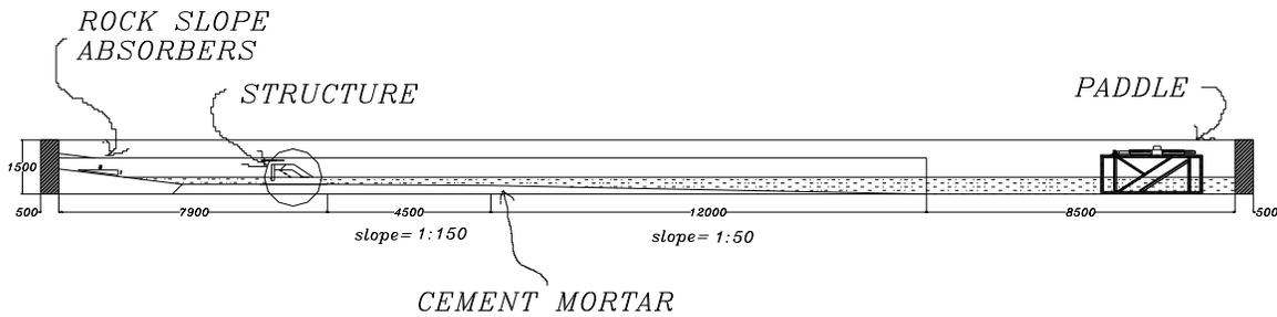
Figure 3: Cross section of the wave flume
