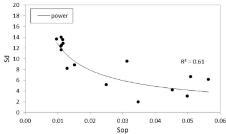
Figure 7: Damage parameter diagram against maximum wave steepness
