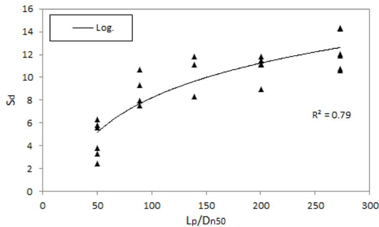
Figure 6: Damage parameter diagram against maximum length wave
