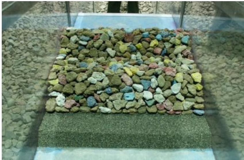
Figure 4: Physical modeling of berm reshaping seawall
