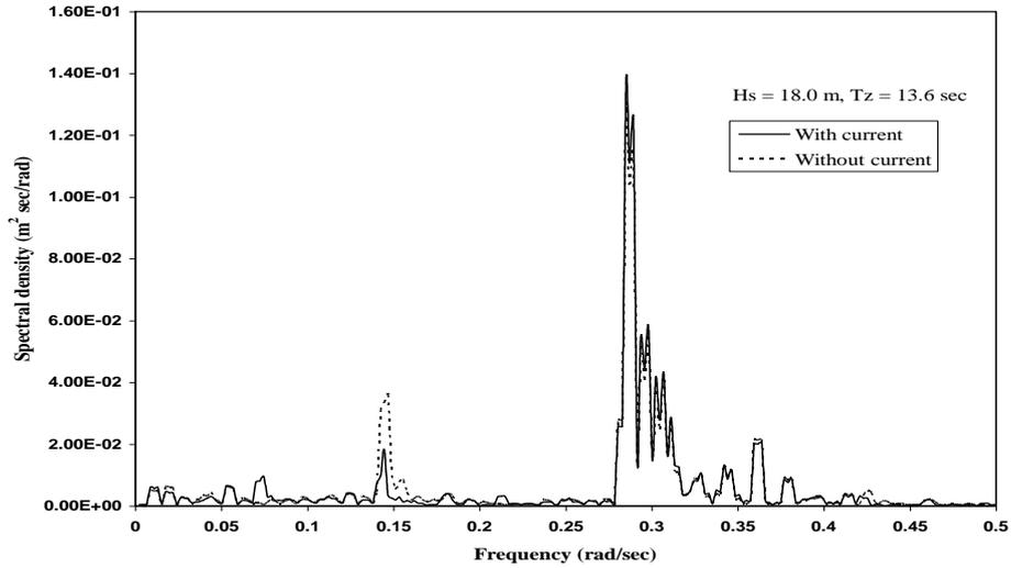
Fig. 3. PSD of surge response under large sea state
