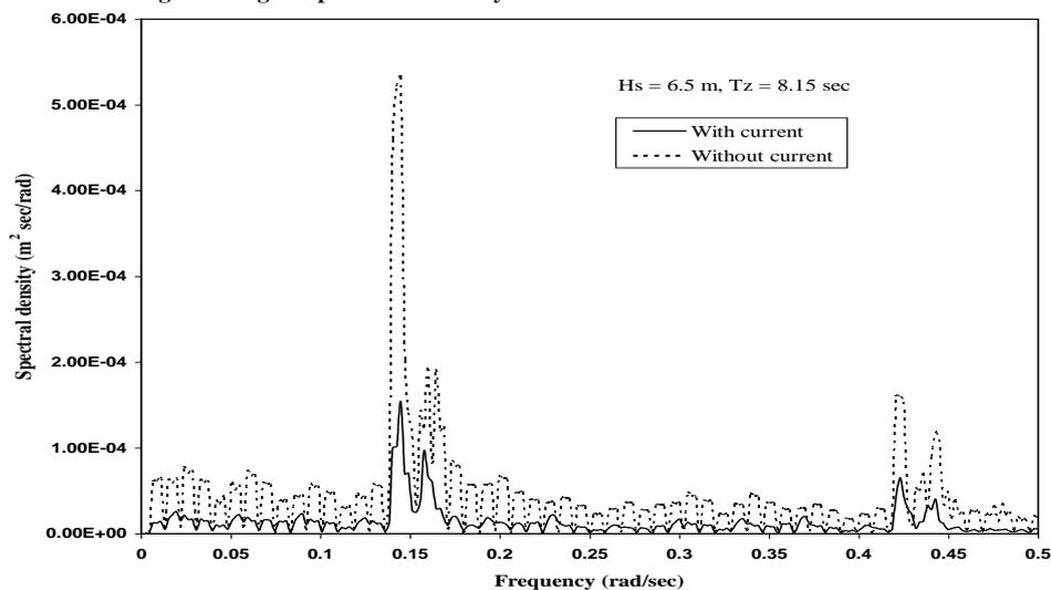
Fig. 11. PSD of surge response under moderate sea state
