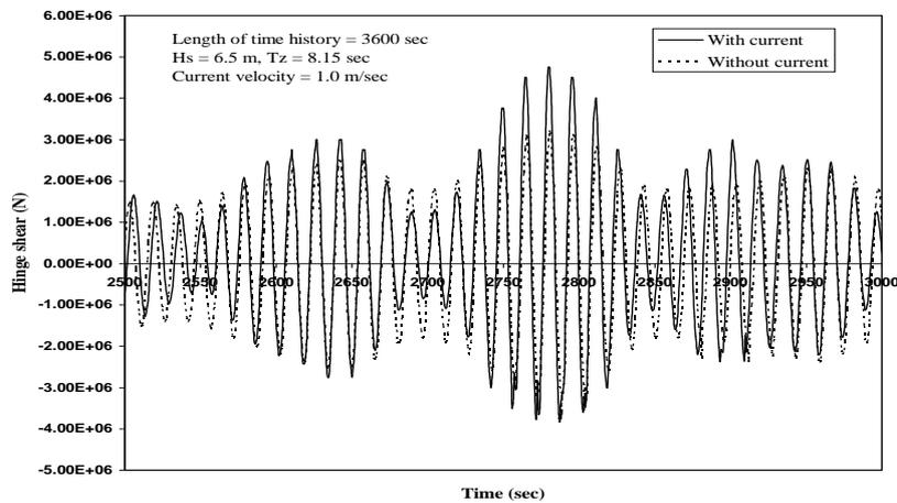
Fig. 14. Central hinge shear response time history under moderate sea state
