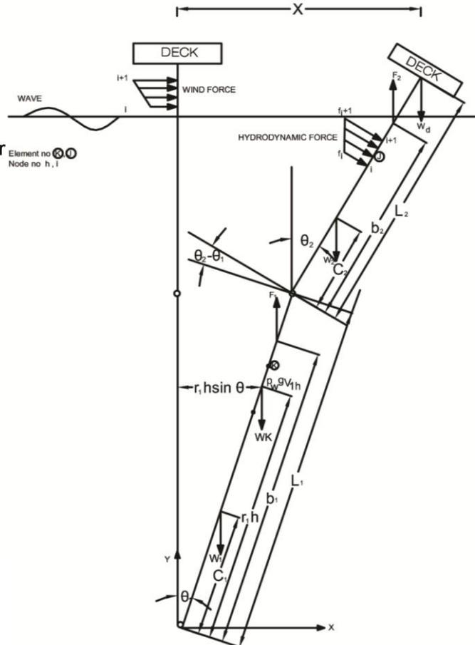
Fig. 1(b) Schematic of double hinged articulated tower
