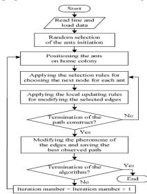
Fig 3: Flowchart of DG using ACO
