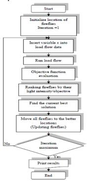
Fig 2: Flow of optimal allocation of DG using FA
