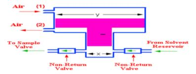
**Displacement pump (Syringe pump):** It produces a flow that tends to be independent of viscosity and back pressure and also the output is pulse free. But it possesses a limited capacity (250 ml). For micro-HPLC applications, a syringe pump allows for the maintenance of a constant flow at the microliter per minute flow rate range. The syringe pump has to be refilled after it displaces the whole syringe volume (Figure 7). **Figure 7.** Syringe pump for high performance liquid chromatography.
