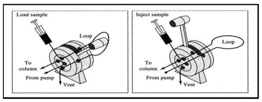
Figure 11. Inject (move the sample loop into the mobile phase flow).
