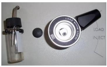
Figure 9. Redone injectors for high performance liquid chromatography.
