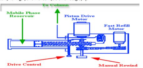
**Reciprocating pump:** It has a small internal volume (35 to 400  $\mu$ l), a high output pressure (up to 10,000 psi), and constant flow rates. But it produces a pulsed flow (Figure 8) <sup>[10-12]</sup>.
