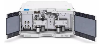
**Pneumatic or constant pressure pump:** They are pulse free; suffer from limited capacity as well as a dependence of flow rate on solvent viscosity and column back pressure. They are limited to pressure less than 2000 psi (Figure 6). **Figure 6.** Pneumatic pump for high performance liquid chromatography.
