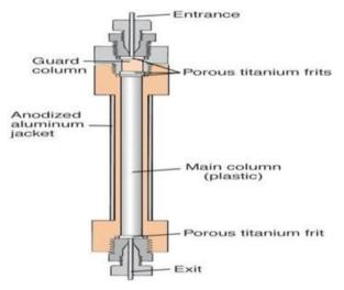
Figure 13. Construction of high-performance liquid chromatography column.
